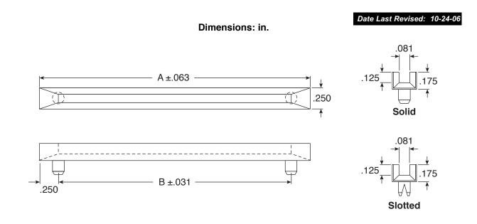
Printed circuit board support guides are an economical and fast solution to mount P.C. Boards. Card insertion is simple and fast. The smooth positive channel guides the P.C. Board and firmly supports and protects the board. Guides are molded of tough, electrically insulating nylon 6/6 and are designed to snap into pre-punched holes in the chassis.
